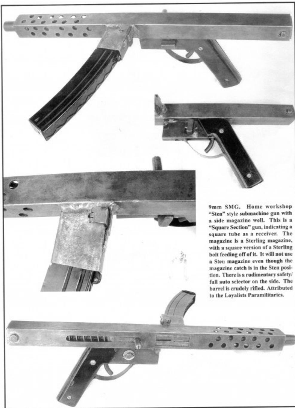
9mm SMG. Home workshop "Sten" style submachine gun with a side magazine well. This is a "Square Section" gun, indicating a square tube as a receiver. The magazine is a Sterling magazine, with a square version of a Sterling bolt feeding off of it. It will not use a Sten magazine even though the magazine catch is in the Sten position. There is a rudimentary safety/full auto selector on the side. The barrel is crudely rifled. Attributed to the Loyalists Paramilitaries.
