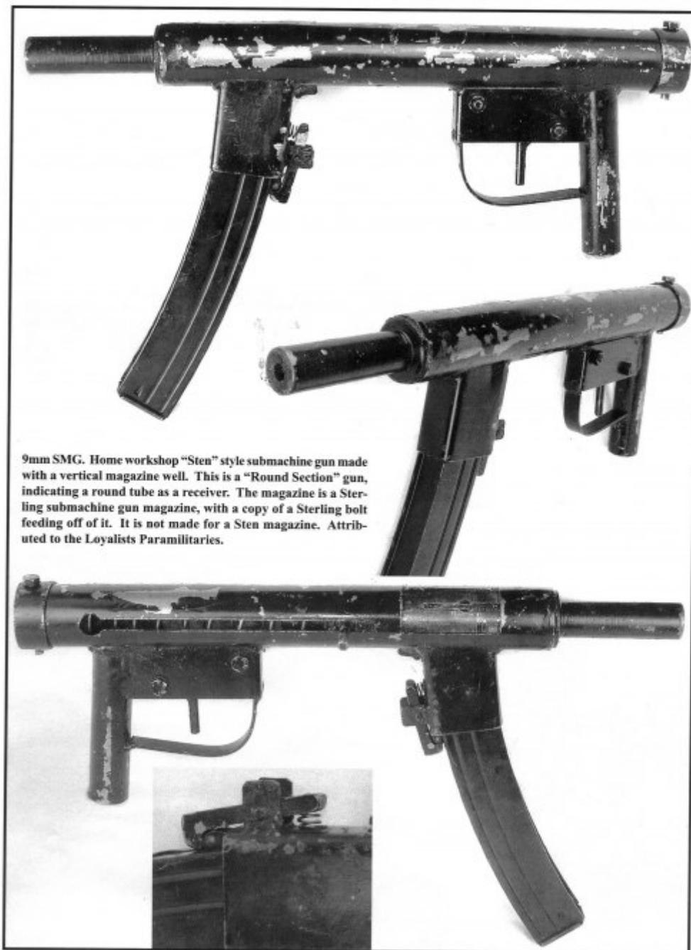
9mm SMG. Home workshop "Sten" style submachine gun made with a vertical magazine well. This is a "Round Section" gun, indicating a round tube as a receiver. The magazine is a Sterling submachine gun magazine, with a copy of a Sterling bolt feeding off of it. It is not made for a Sten magazine. Attributed to the Loyalists Paramilitaries.
